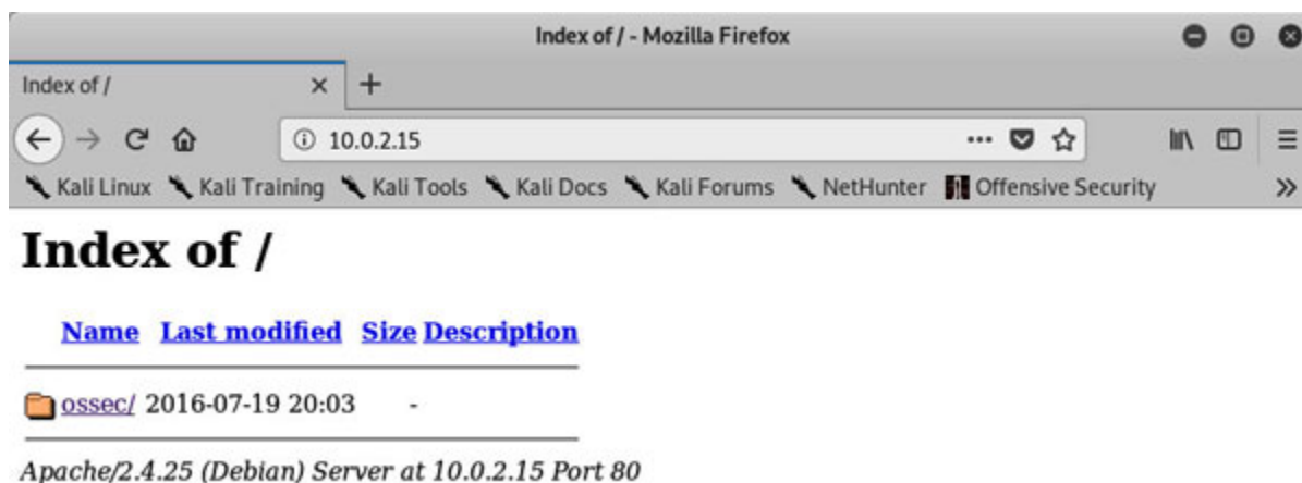
Figure 6.11: HTTP service running on port 80
